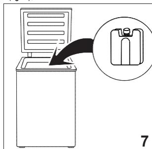
6. Put the ice box/pack vertically in the front left corner of the tank as shown in figure 8;
