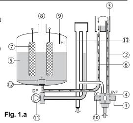
As the water fills the cylinder, it will reach the electrodes (7) and current will begin to flow. As the water continues to fill the cylinder, the current will
