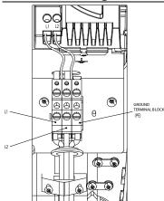
Check that the power supply voltage to be connected matches the value indicated on the rating plate inside the electrical panel.
