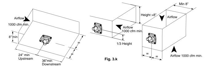
IMPORTANT: Allow 1 M ( 3 feet ) of straight duct downstream of the distributor pipes and nozzles for absorption of the steam. Always allow 0.6M (2 feet) of straight duct upstream of the distributor pipes for evaporation of the steam. Turbulent air flow may require longer lengths.
