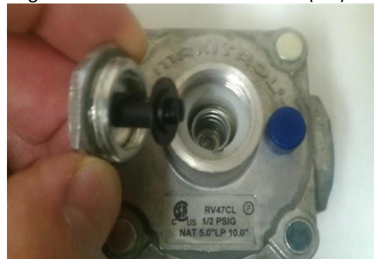
Regulator Converted to Liquid Propane (LP)
