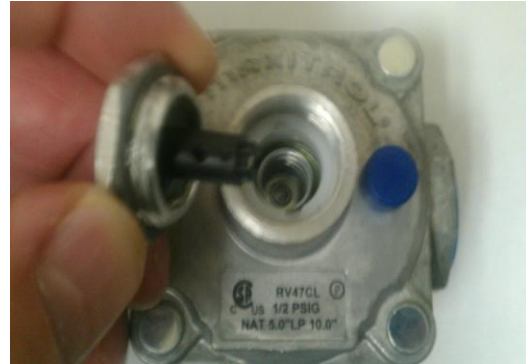
Regulator Converted to Natural Gas (NG)
