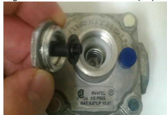
Regulator Converted to Liquid Propane (LP)
