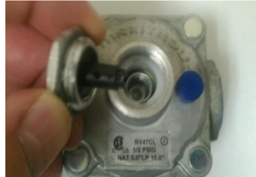
Regulator Converted to Natural Gas (NG)
