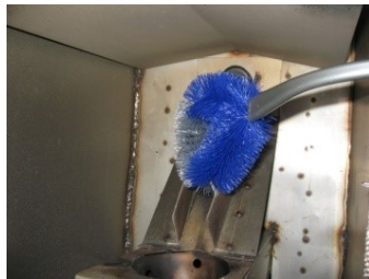
Figure 2: Pellet Slide Cleaning
