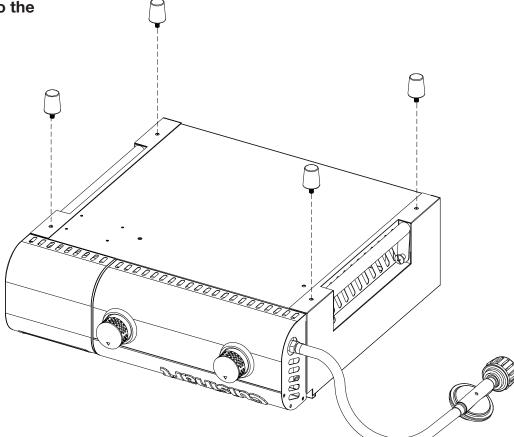
**Step 3:**Put the griddle top on the griddle body. Make sure stand offs of each corner on the griddle top's bottom is aligned and seated on the griddle body.
