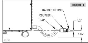
• Screw the supplied hose barb fitting into the coupler and attach the supplied 1/2 inch I.D. drain hose. Route the hose to the nearest drain.
