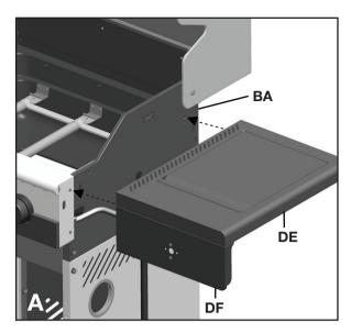
a. Open the lid. Assemble the Right Side Shelf (DE and DF) to the Cart Assembly by inserting the Side Shelf tabs into the holes on the Cart Assembly, as shown in figure A.
