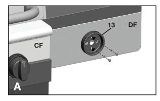
a. Assemble the Side Burner Control Knob Bezel (#13) to the Right Side Shelf Fascia (DF) as shown in figures A.
