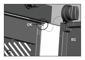
a. Assemble the Door Assembly (EC), to the Bottom Shelf (ED) by inserting the fixed pin (bottom of door) into the hole provided as shown in Figure B.
