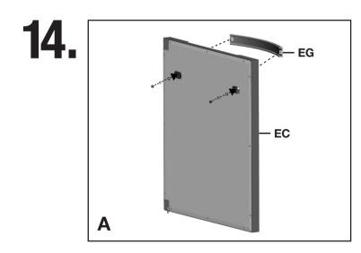
Assemble the Door Handle (EG) to the Door Assembly (EC) as shown in Figure A.
