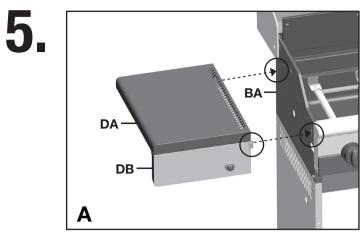
a. Open the lid. Assemble the Left Side Shelf (DA and DB) to the Cart Assembly by inserting the Side Shelf tabs into the holes on the Burner Box Asembly (A and B).
