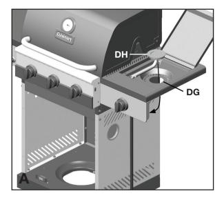
a. Position the Side Burner (DH) through the opening in the Side Burner Drip Pan (DG).
