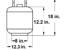
**A** The LP cylinder used must include a collar to protect the cylinder valve.
