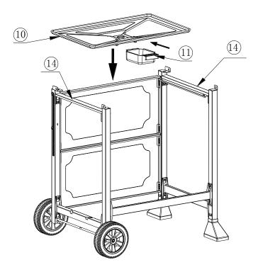
8. Require two people to lift and place the Firebox Assembly onto the cart and fasten 4pcs AA Screws as shown.
