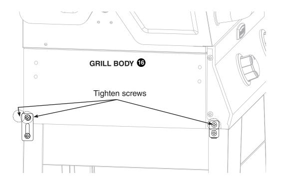
Tighten 3 screws (Removed in Step 13)
