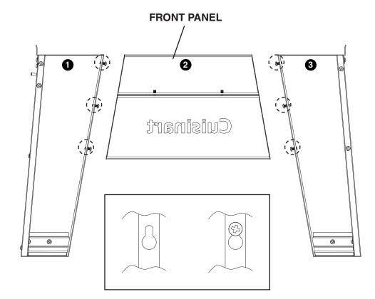
**NOTE:** Before tightening keyhole screws, make sure panels are aligned.
