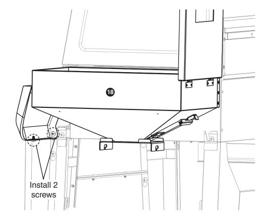
Install PELLET HOPPER LID HANDLE (screws, washers and bezels are pre-installed in handle)
