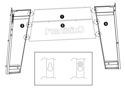
**NOTE:** Before tightening keyhole screws, make sure panels are aligned.
