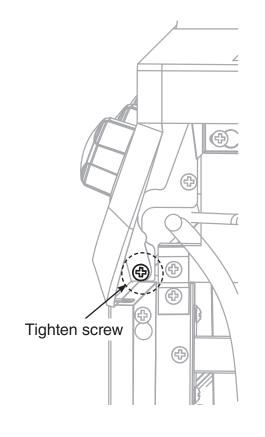
Install screw and tighten (screw was removed in Step 12)
