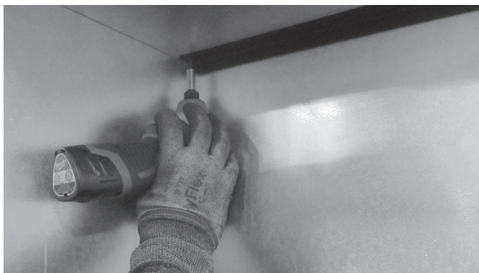
Figure 7.2 - Remove Rear Black Magic Glass Bracket
