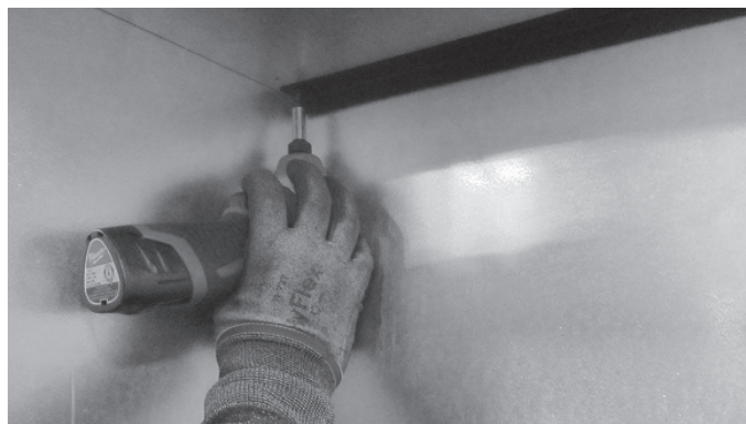
Figure 7.2 - Remove Rear Black Magic Glass Bracket
