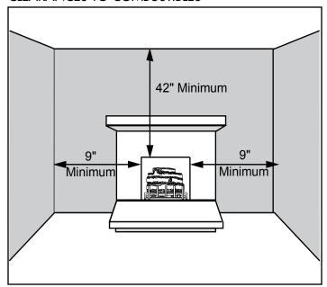
**Back Wall Clearance** — The appliance may be placed against a combustible back wall.
