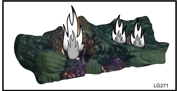
Fig. 45 Correct burner flame appearance for 33BDVR.
