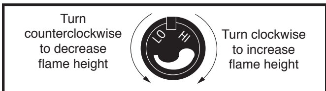
Fig. 51 Flame adjustment knob for Honeywell valve.
