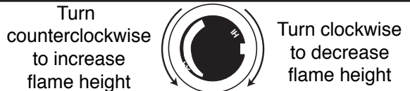
Fig. 55 flame adjustment knob for SIT valve.
