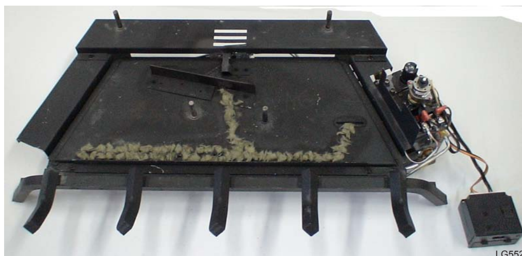
Figure 19 - Correct Rock Wool Placement
