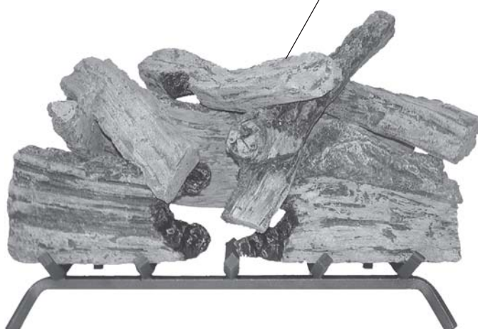
Figure 109 - Installing Top Center Log (#7)
