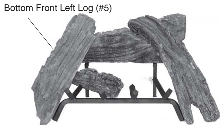
Figure 71 - Installing Bottom Front Left Log (#5)
