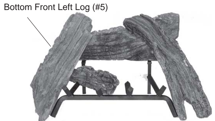
Figure 71 - Installing Bottom Front Left Log (#5)
