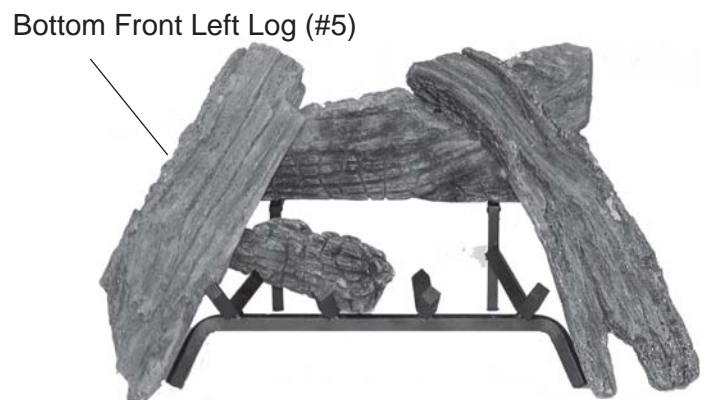
Figure 71 - Installing Bottom Front Left Log (#5)
