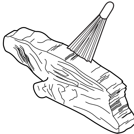
Figure 152 - Removing Soot with a Soft Bristle Brush
