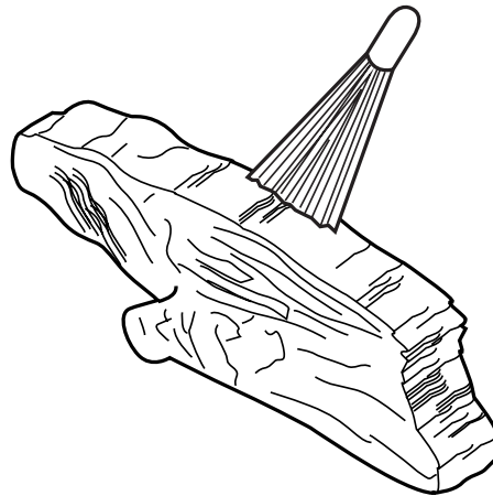
Figure 152 - Removing Soot with a Soft Bristle Brush
