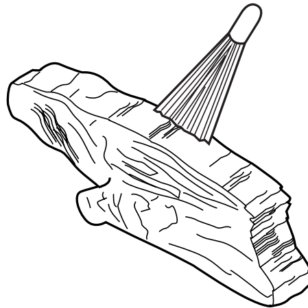
Figure 152 - Removing Soot with a Soft Bristle Brush
