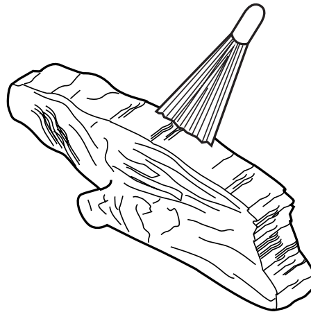
Figure 152 - Removing Soot with a Soft Bristle Brush
