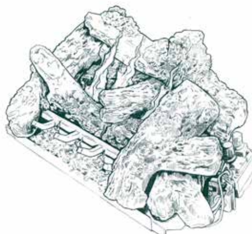
Figure 5.21 - Correct Appearance of Rear Flames
