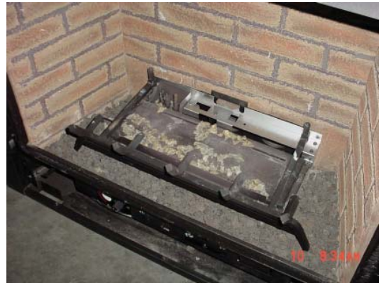
Figure 46 - Placement of Rock Wool on Burner
