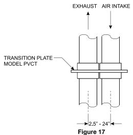
clearances between intake and exhaust pipes.
