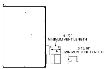
Step 5. Slide co-axial vent pipes into co-axial adaptor.
