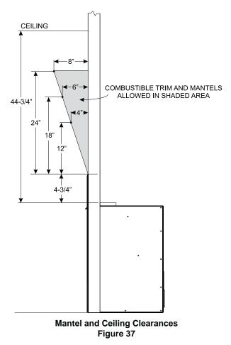
**Note:** The Mantis Power-Vent High-Efficiency Fireplace has been tested and approved for zero clearance to combustible materials. It is recommended that clearances as listed above should be maintained to allow for removal of the product for servicing.
