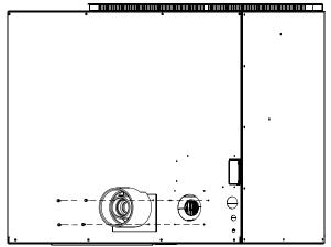
**Step 2.** Attach co-axial direct vent adaptor and gasket (4 screws) to the rear of fireplace.
