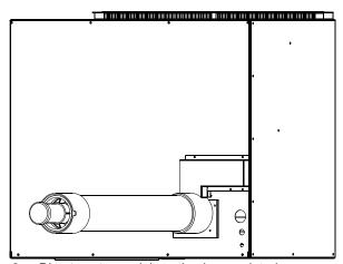
Step 6. Direct vent co-axial venting is completed.
