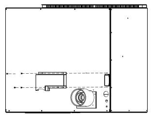
**Step 3.** Attach co-axial air-inlet duct to rear of fireplace (6 screws).
