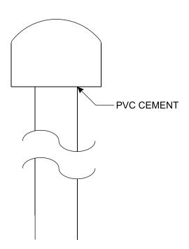
PVVTC Vertical exhaust cap used with 1 1/2" PVC pipe installation. Termination cap can also be used with colinear transition plate model PVCT. Refer to Figures 10-13, 15, 19 and 20 for venting examples.
