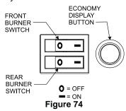
To use this feature, both burner switches need to be in the "ON" position, and the red button must be pressed so it is illuminated. This will ignite the front burner. The front burner will remain on when the red button is illuminated, and the back burner will cycle with the thermostat. The red button acts only as an override for the front burner.
