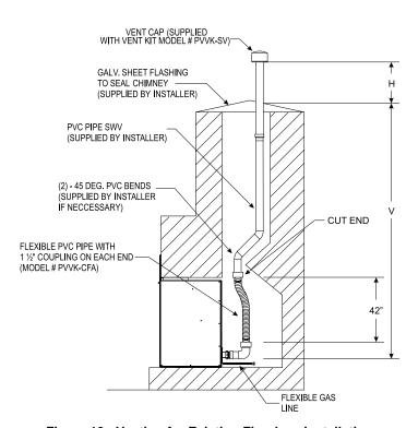
Figure 10 - Venting for Existing Fireplace Installation
