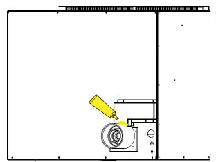
**Step 4.** Install silicone around connection between co-axial adaptor and co-axial air-inlet duct.
