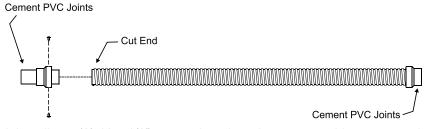
Once length is determined, install two (2)  $10 \times 1/2$ " screws into the adaptor assembly to secure the adaptor assembly to the flex hose. Using PVC cement, cement all PVC joints of the flex vent kit to the remaining PVC vent run.
