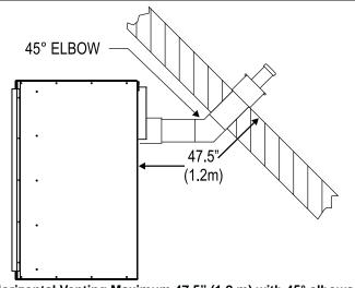
Horizontal Venting Maximum 47.5" (1.2 m) with 45° elbows. Inner 1-1/2 inch pipe and outer 3 inch pipe 45° elbows can be purchased from a local hardware store.
