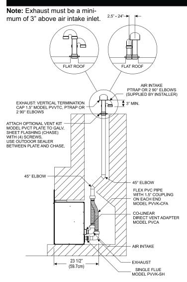
Colinear Direct Vent - Insert Installation Figure 18
