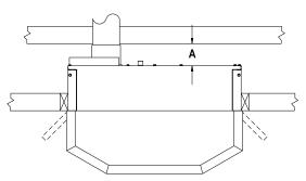
**Co-axial Venting Installation Shown** Single Flue requires surround for combustion air. Figure 32
