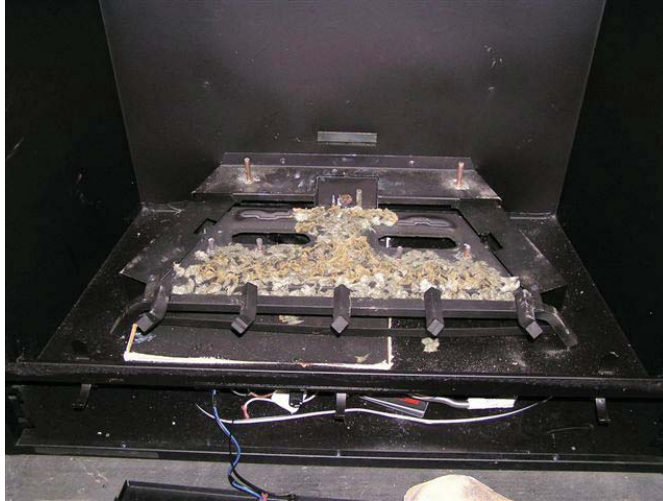
Figure 45 - Rock Wool Placement on Rear of Burner.
