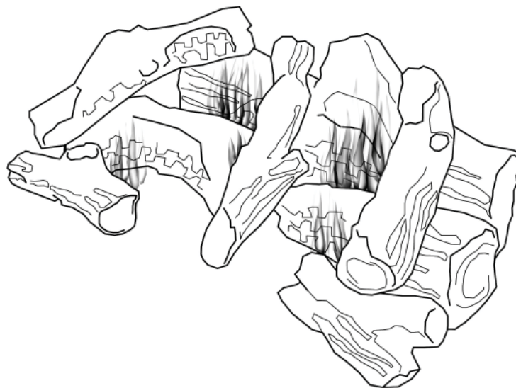
Figure 61 - Burner Flame Appearance
