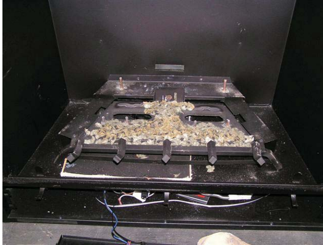
Figure 45 - Rock Wool Placement on Rear of Burner.
