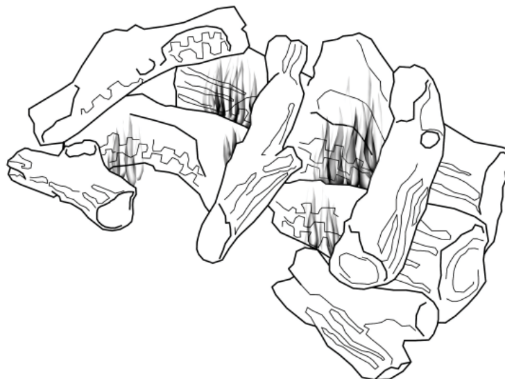
Figure 61 - Burner Flame Appearance
