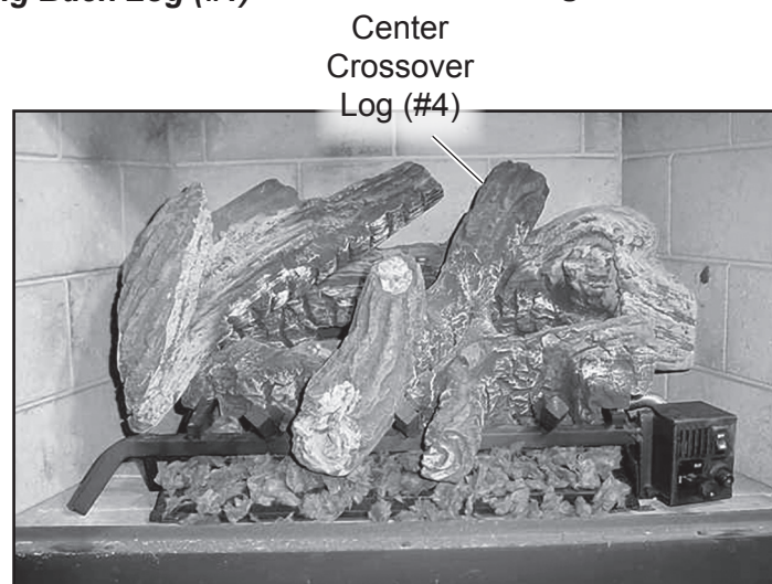
Figure 16 - Placing Center Log (#4)
