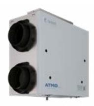
Fantech's, ATMO 150E is an Energy Recovery Ventilator designed for higher static pressure applications. The unit brings a continuous supply of fresh air into a home while exhausting an equal amount of contaminated air. The energy recovery core at the center of the unit transfers heat and moisture from incoming air to the outgoing air that was cooled and dried by the building's air conditioner.
