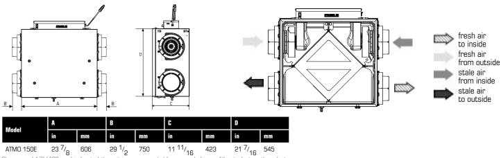
Clearance of 17" (432 mm) in front of the unit is recommended for removal of core. All units feature three foot plug-in power cord with 3-prong plug.
