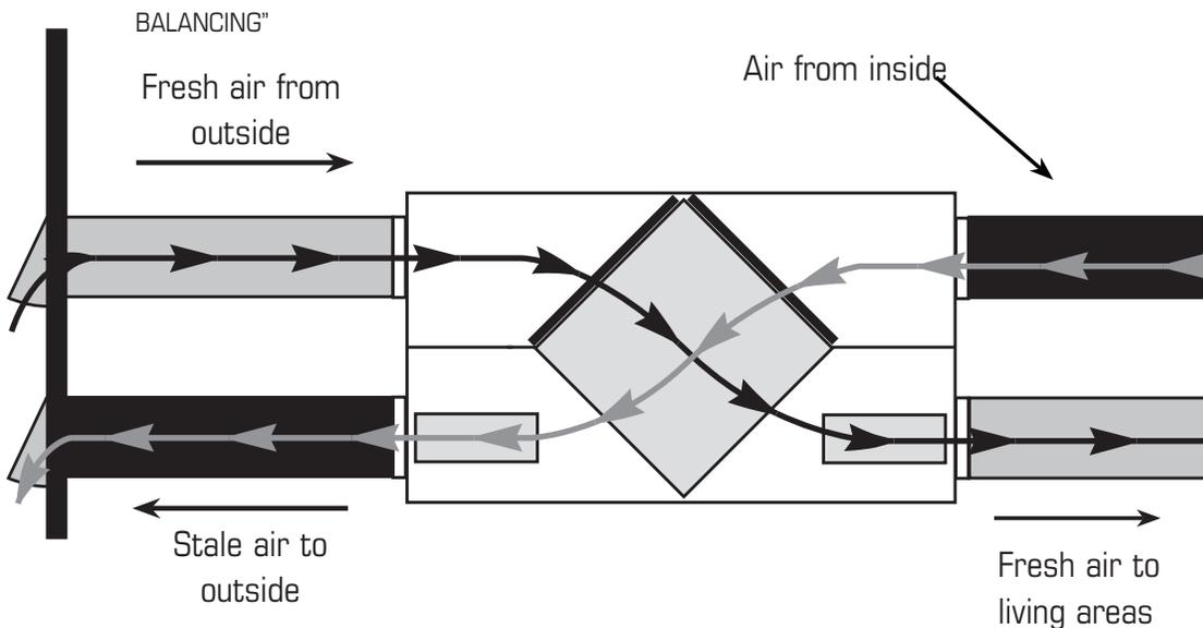
\* Unit air flow should be balanced while FAA is on "Normal" speed and furnace blower is running.
