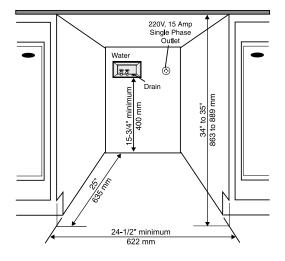
If the drain outlet is higher than 24", the connections will need to be recessed.
