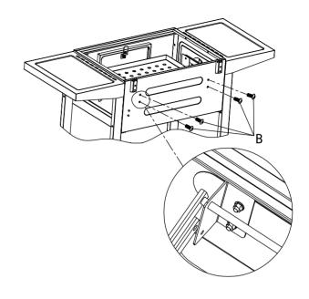
Fasten the charcoal pan attached to the rear panel with 4 bolts (B).
