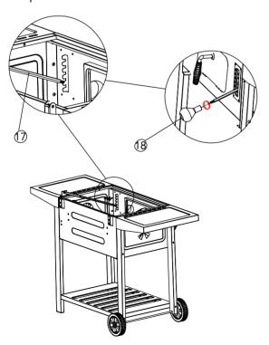
Twist the lever knob (18) onto the lever (17) as shown.
