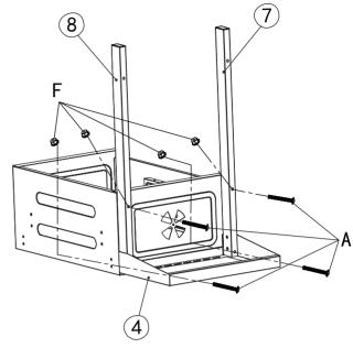
Assemble the right front leg (7), the right back leg (8), and the side table (4) to the right side panel with 4 bolts (A) and 4 nuts (F). Please note: Don't secure and tighten all the bolts until step 5.
