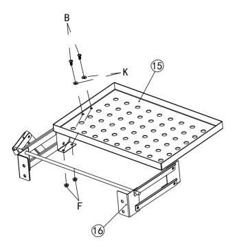
Assemble the charcoal pan (15) and the charcoal pan brace (16) with 4 bolts (B), 4 washers (K) and 4 nuts (F) as shown, and (K) must be inserted between (B) and (F).
