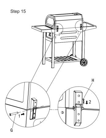
Connect the lid with the firebox by securing hinges with 2 hinge pins (G) and 2 split pins (H).
