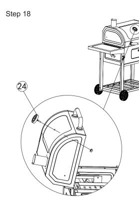
Insert the thermometer (24) into the lid and secure it in place by using a nut.
