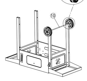
Slide axle (10) through the left legs. Attach the wheel washers (I) and wheels (11) to both ends of the axle. Secure each wheel with a split pin (C).
