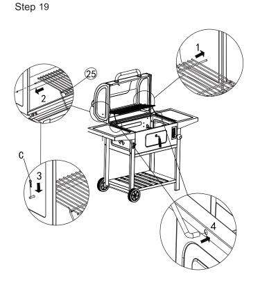
Insert the warming rack (25) by attaching it to the firebox and the lid. Secure it with 2 split pins (C).
