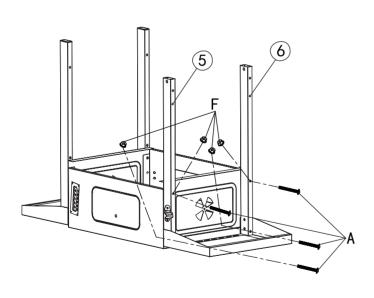
Assemble the left front leg (5), the left back leg (6), and the side table (4) to the left side panel with 4 bolts (A), and 4 nuts (F).
