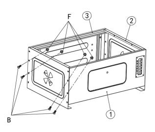
Assemble the two side panels (2), the front panel (1) and the rear panel (3) with 8 bolts (B) and 8 nuts (F). Please note: Screw the bolts into the second and the third screw-holes.
