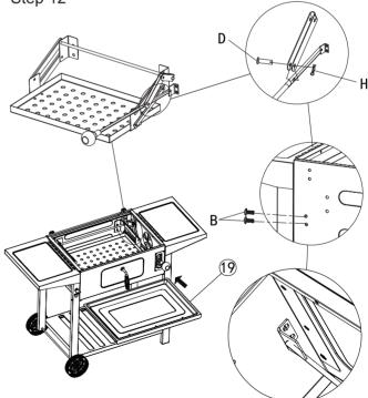
Secure the lever (17) by using 1 split pin (H) and 1 hinge pin (D) to the right side of the charcoal pan lifting system. Secure the lever (17) to the rear panel with 2 bolts (B).
