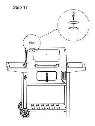
Assemble the cover to the stack, screw back the bolt as shown.
