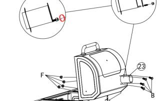
Loosen the bolt on the stack (23), and take off the cover. Then assemble the stack (23) to the lid with 4 bolts (B) and 4 nuts (F).
