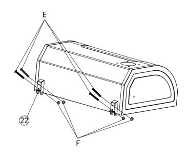
Fasten the upper hinges (22) to the lid with 4 bolts (E) and 4 nuts (F).
