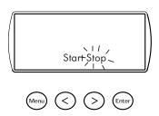
The program has stopped temporarily because the door has been opened, the main power switch has been turned off or the power supply has been interrupted.
