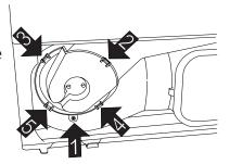
4. Unscrew the nut while holding the fan.
