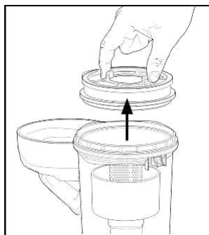
3. Remove the dust cup foam filter.
