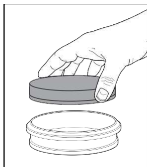
5. Allow filter to dry 24 hours before putting back into vacuum cleaner.
