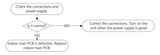
Note: E2 zero crossing detection error is only valid for the unit with AC fan motor, for other models, this error is invalid.
