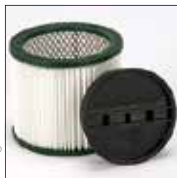
90341 (TYPE II) Small CleanStream® HEPA Cartridge Filter 99.97% efficient down to 0.3 microns. Non-stick surface makes for easy clean up and resists clogging. Fits 1-4 U.S. gallon vacs 5 U.S. gallon portable model H87S, 5 U.S. gallon HangUp®/ Wall Mount vacs and 6 U.S. gallon long life model P12S. Does not fit 1x1® Micro®, HangOn® and HangUp® Mini.
