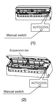
**NOTE:** The unit must be turned off before operating the manual control button. If the unit is operational, continue pressing the manual control button until the unit is off.
