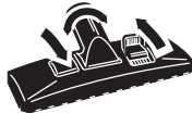
Dual Surface Selector Nozzle Levers control brush position for various types of cleaning.
