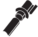
All Friction Fit Wands Insert wand ends together and twist to form a tight fit.
