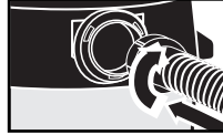
All Friction Fit Hoses Insert machine hose end into tank and twist to form a tight fit.
