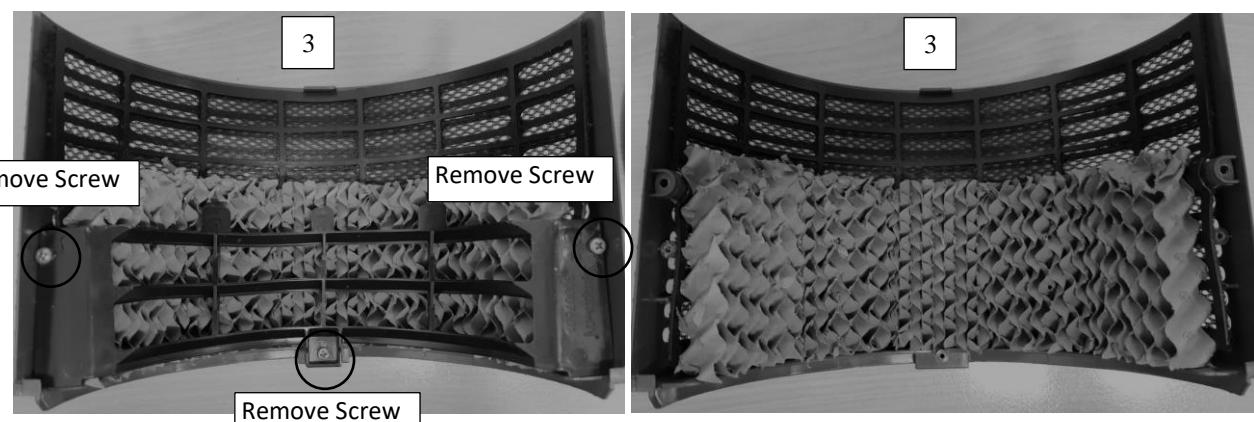
4- Assemble in reverse order, ensuring the panels are fitted correctly with no gaps or tabs left outside.
