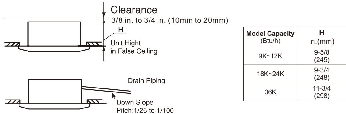
Fig. 3.2 Installation Location of Indoor Unit
