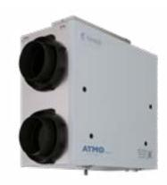
Fantech's, ATMO 200E is an Energy Recovery Ventilator designed for higher static pressure applications. The unit brings a continuous supply of fresh air into a home while exhausting an equal amount of contaminated air. The energy recovery core at the center of the unit transfers heat and moisture from incoming air to the outgoing air that was cooled and dried by the building's air conditioner.
